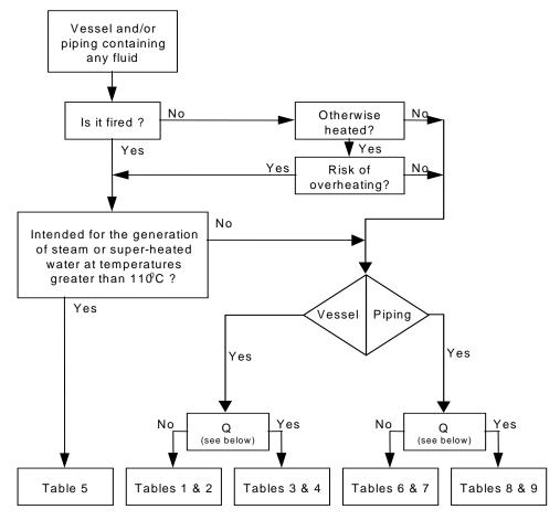
Q.Does the vessel or piping contain liquid whose vapour pressure at the maximum allowable temperature is not more than 0,5 bar above normal atmospheric pressure?
