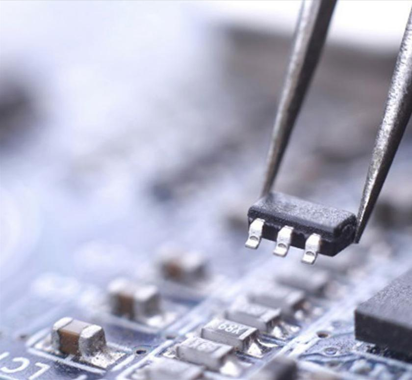
A close-up photograph showing a pair of tweezers holding a small, dark, rectangular microchip with three pins. The chip is being positioned over a printed circuit board (PCB) which has various other components and traces visible. The background is blurred, focusing attention on the chip and tweezers.
