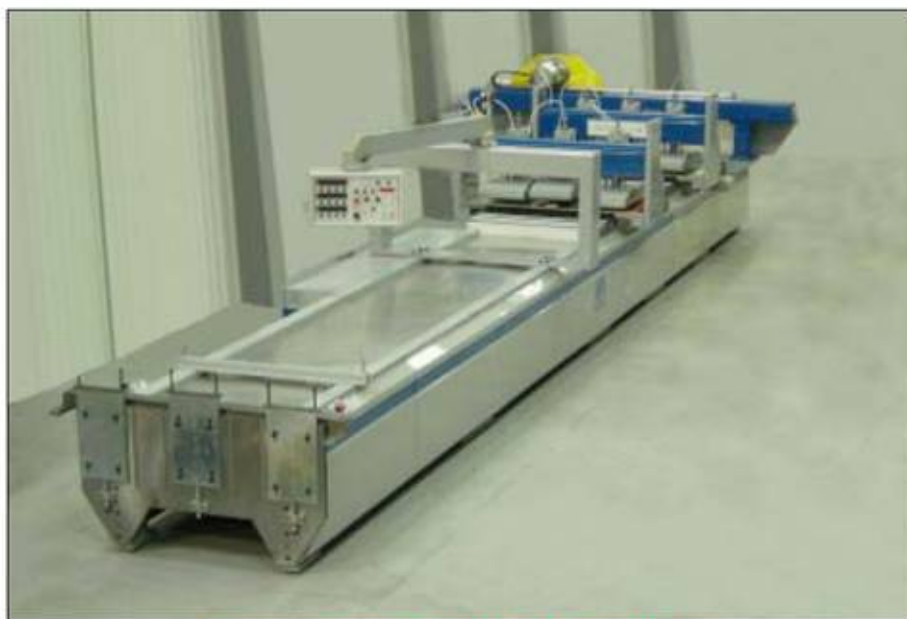
4 clamp modules on the Px 1400-24T Pultrusion Machine
