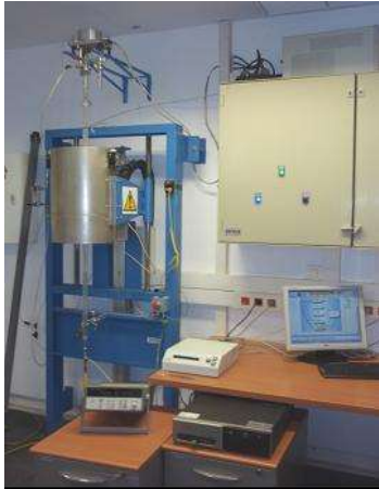
Multicycle testing TG at CSIC
